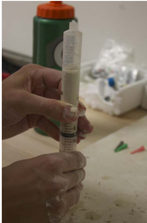
Figure 26: Pushing clay from loader to syringe.
