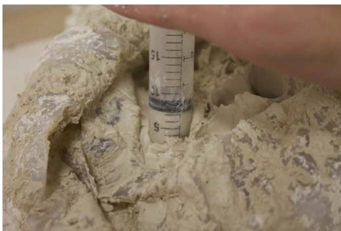
Figure 24: Sucking clay into the loader.
