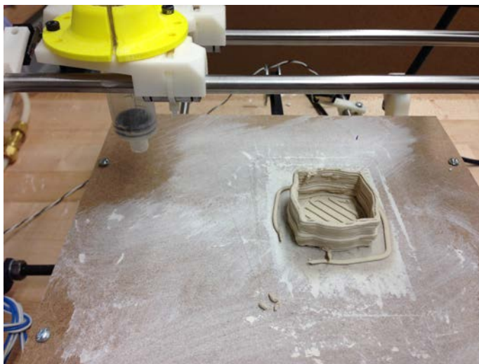
Figure 30: A small object printed directly on the MDF printbed.
