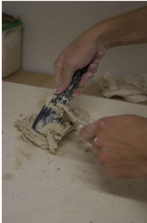
Figure 22: Mixing clay paste with putty knives.
