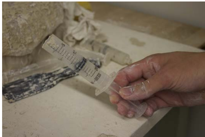
Figure 23: An empty clay loader, made from a modified syringe.
