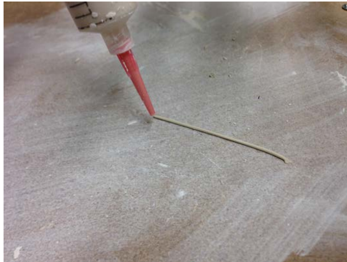
Figure 28: Calibrating the feedrate by extruding for periods of 1 second.
